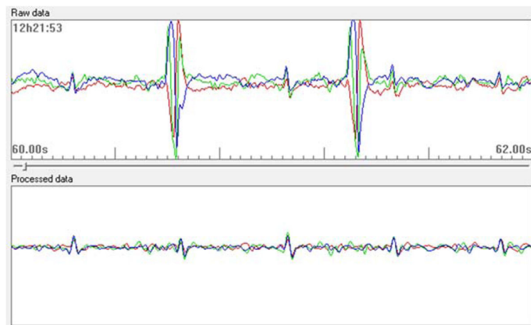
Figure 1. Sample of Monica AN24 abdominal monitor raw signal. This sample demonstrates the raw fetal ECG data obtained from the monitor with each color representing output from a different electrode.
