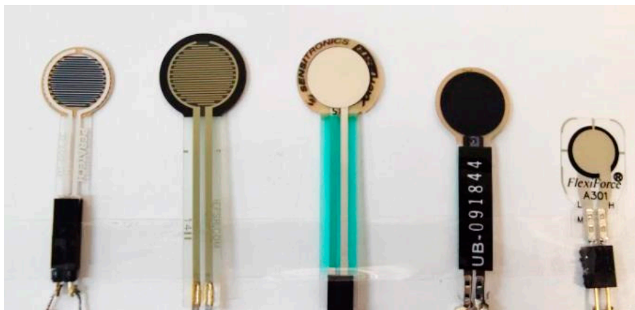
Figure 1. Evaluated force sensing resistors (left to right): Peratech QTC™, Interlink FSR®, Sensitronics® FSR, Tactilus® Sensor and Tekscan Flexiforce® A301.
