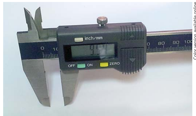
Fig. 1. The digital caliper (Terensa, USA) used for the measurement of the ICA between the upper anterior teeth.
