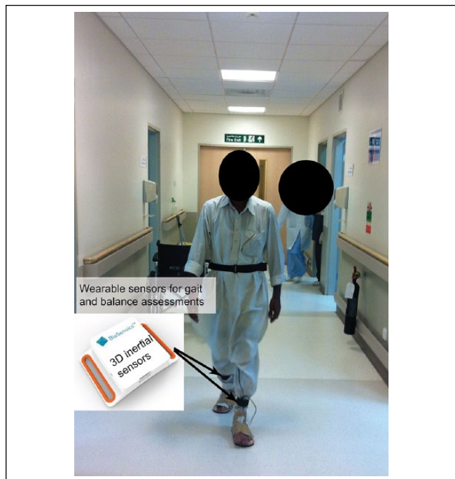
Figure 2. Patients during assessment of postural balance and gait in a clinical setting. Body-worn sensors attached to shank, thigh, and lower back for assessment of postural balance.
