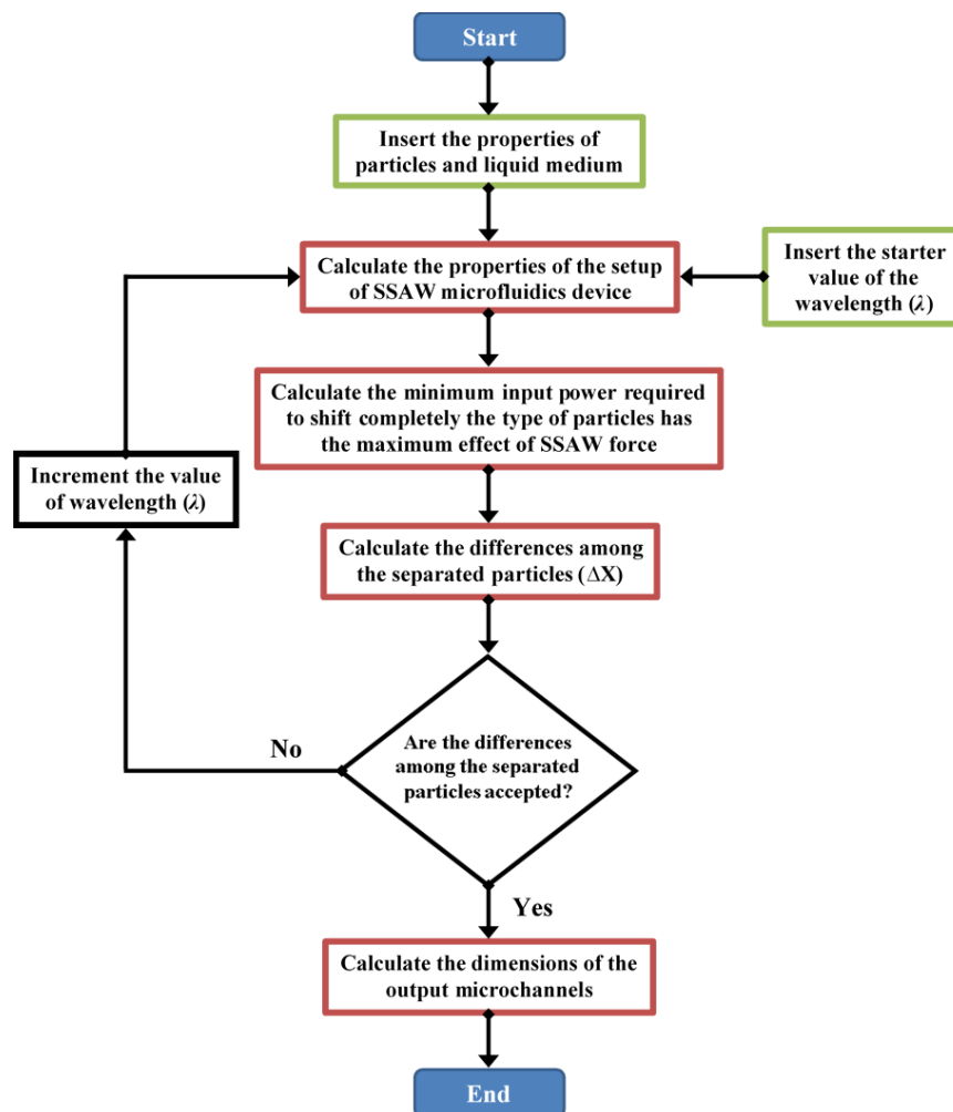
Figure 4. The flow chart of proposed design analysis of SSAW microfluidics for specific separation process.
