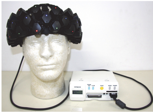
Fig. 3 Photograph of wearable fNIRS system using LED and APD modules.
