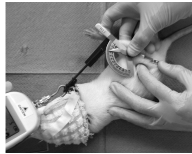
Fig. 2. Measurement of range of motion The knee joint ROM was measured by goniometer for use in finger with original attachment. The knee joint was pulled in 0.04Nm by tension meter.
