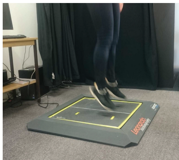
Supplementary Figure S1. Leonardo Mechanograph Ground Reaction Force platform used for jumping and hopping assessments in the VIBE Study. Here two-legged counter-movement jump (2LJ) is demonstrated.
