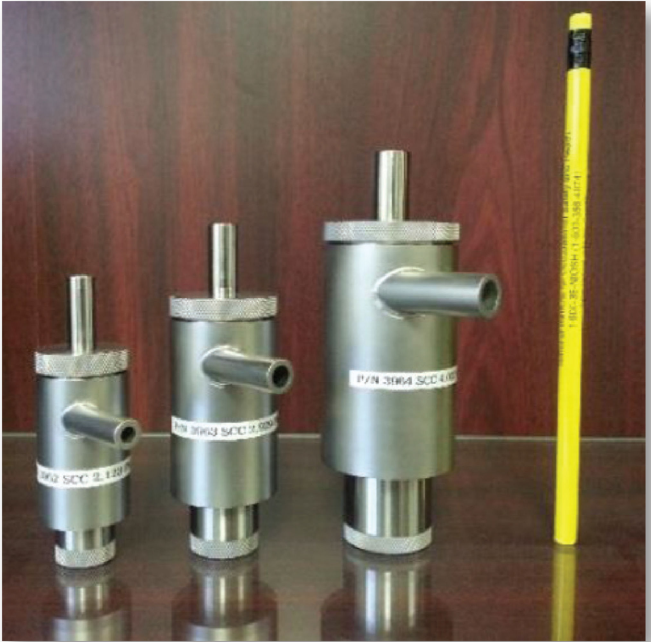
Figure 2. Custom-cut cyclones: 10, 20 and 40 \mu\text{m} .
