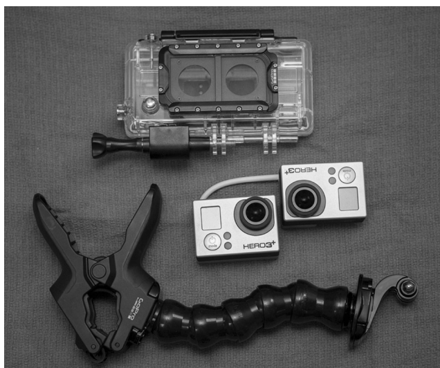
Fig. 1 Two GoPro HERO 3+ Black Edition cameras and the Dual HERO System housing
