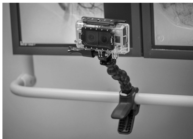
Fig. 2 GoPro cameras mounted on the video boom with the GoPro Jaws Flex Clamp
