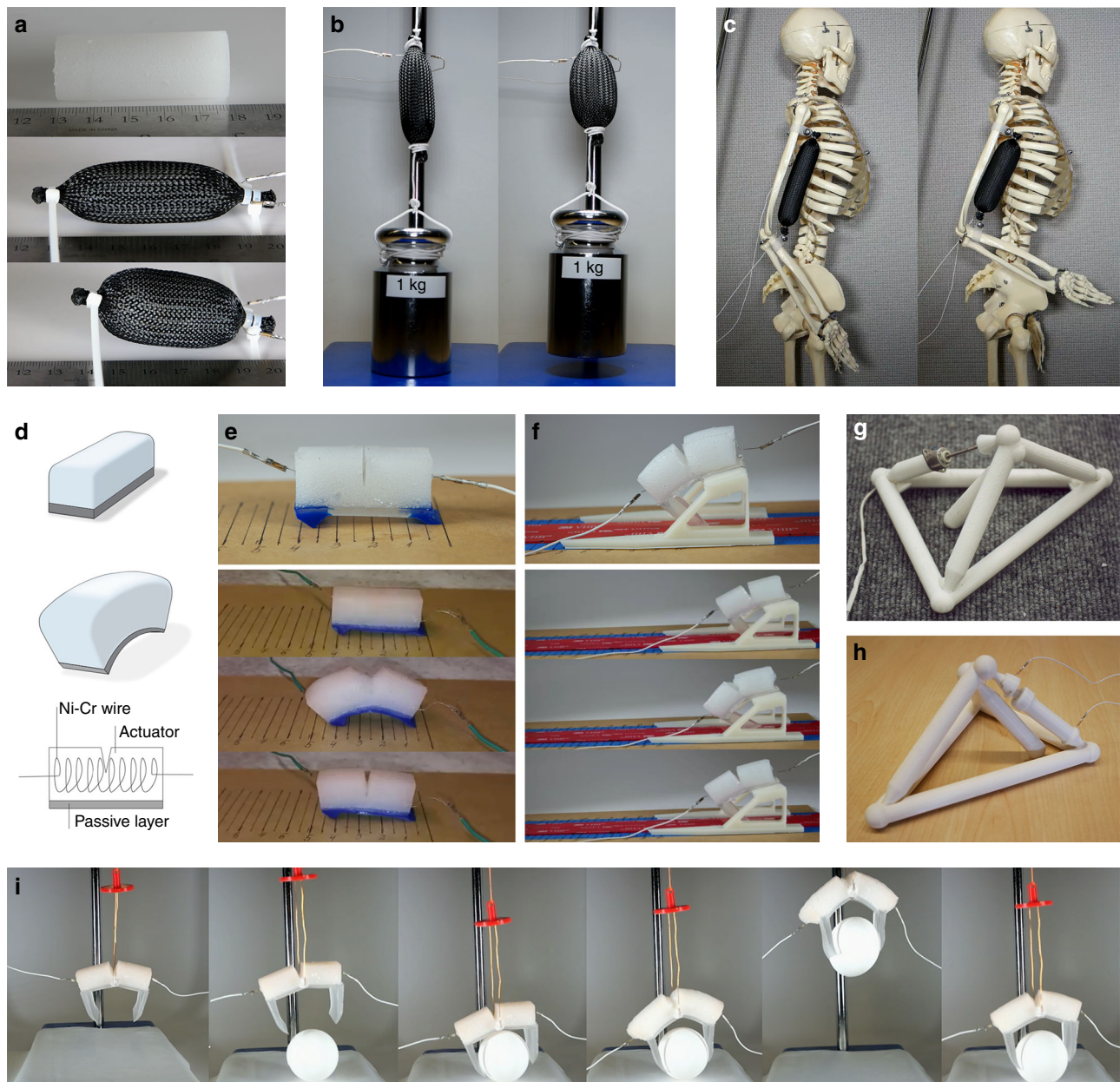
Fig. 4 Implementation of the soft composite material as an actuator. a McKibben-type artificial muscle (soft composite material inside braided mesh sleeving) shows displacement of about 25%. b 13 g artificial muscle lifts the weight of 1 kg. c Soft artificial muscle implemented as a biceps lifting skeleton's arm to 90° position at elbow ( a–c : actuation powered at 45 W (30 V, 1.5 A)). d Design of the bi-morph bending actuator. e All-soft two-leg “worm” and its locomotion powered at 8 W (8 V, 1 A). f The sleigh robot and its locomotion powered at 8 W (8 V, 1 A). g Tetrahedral robot evolved and 3D-printed in 2000 34 with embedded electrical motor. h The same robot with the soft composite material as an actuator embedded instead of the electrical motor. i Soft gripper lifting an egg (sequence from left to right; 8 V, 1 A)
