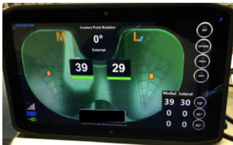
Fig. 3. Left knee. Loading forces at tibiofemoral interface. In this example, the knee is well balanced with 39 lbs in the medial compartment and 29 lbs in the lateral compartment: the intercompartmental load difference is 10 lbs.
