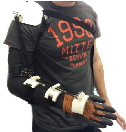
FIGURE 8: Wearable exoskeleton for elbow medical rehabilitation with shape memory alloy actuators.
