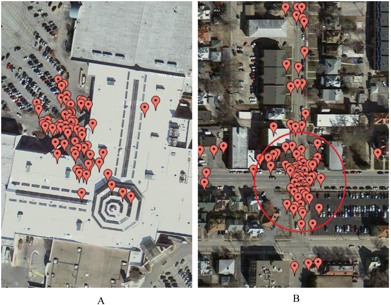
Figure 2. Examples of spatio-temporal cluster (A) and spatio-non-temporal cluster (B). The spatio-temporal cluster shown in (A) reflects a staying activity for which the GPS points were sequentially observed (Note: this is an activity where a subject stayed inside a building for 35 minutes. The subject spent most of the time close to the entrance of the building. The GPS points exhibit a cluster regardless of the temporal sequence). The spatio-non-temporal cluster noted in the red circle in (B) is composed of GPS points that were observed during multiple days when the subject drove past the road intersection. The latter is categorized as a spatio-non-temporal cluster because the GPS points were not sequentially observed and therefore do not fulfill the temporal continuity criterion.
