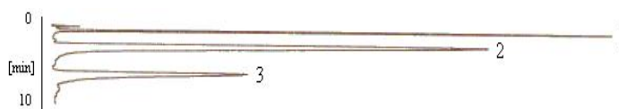
Figure 2. RP-HPLC chromatogram for PER (2), its degradation product (1) and internal standard (3) stored at RH = 76.4%, T = 363 K.
