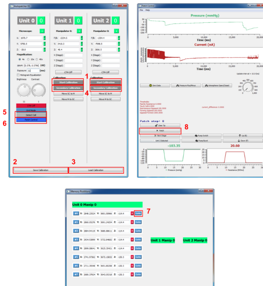
Figure 2. Autopatcher GUI. The buttons mentioned in the protocol are shown in red squares and are numbered. 1: Start Calibration, 2: Save Calibration, 3: Load Calibration, 4: Secondary Calibration, 5: Detect Cell, 6: Patch Control, 7: Go to (target cell coordinate), and 8: Patch. Please click here to view a larger version of this figure.
