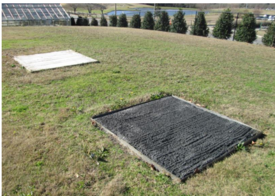
Figure 3. View of Pit with Sand and Pit with 10 Cw% Sand-carbon Mixture. Please click here to view a larger version of this figure.
