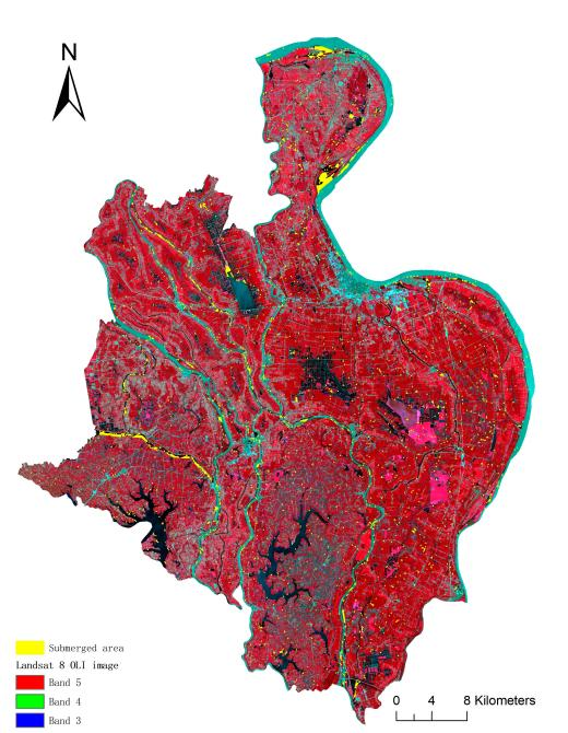
Figure 3. Submerged area.
