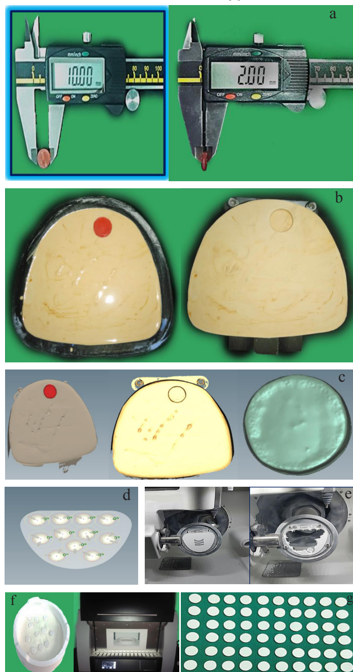
[Table/Fig-1]: Fabrication of Zirconia Discs a) Wax pattern of 10 mm diameter and 2 mm; b) Obtaining master cast of the wax pattern impression; c) Scanning of the pattern using ceramill mind software; d) Scanned pattern nested into zirconia blank for milling; e) Milling of zirconia blank in ceramill motion 2; f) Sintering of zirconia discs in ceramill therm 3. g) sintered 60 zirconia discs.
