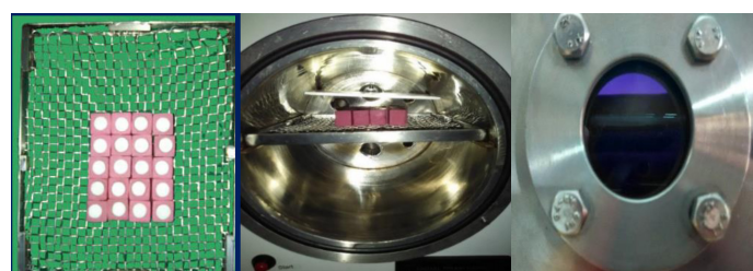
[Table/Fig-3]: Group II samples undergoing plasma of argon cleaning.
