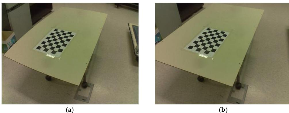
**Figure 5.** Illustrative example for the image calibration algorithm: (a) image distortion resulted from wide-angle lens; and (b) image undistortion using image calibration.
