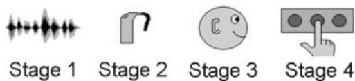
Figure 1 A schematic representing four stages of the listening experience for hearing aid users. Stage 1 includes the incoming signal. Stage 2 addresses the hearing aid and how it modifies the signal. Stage 3 begins when the amplified signal is delivered to the ear and includes transduction and processing by the auditory system. Stage 4 includes higher-order processes up to and including a behavioral response of some kind.
