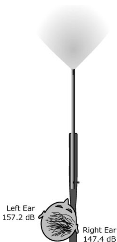
Figure 3 Illustration of head-shadow effect contrasting sound pressure levels measured for each ear for a right-handed rifle or shotgun shooter.
