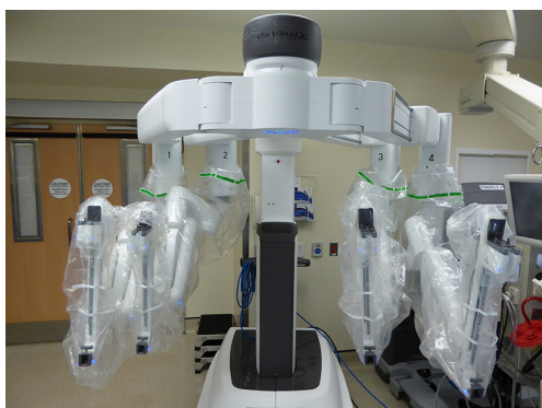
Figure 1 da Vinci™ Xi patient cart is sterilely draped and ready to be deployed over the patient.
