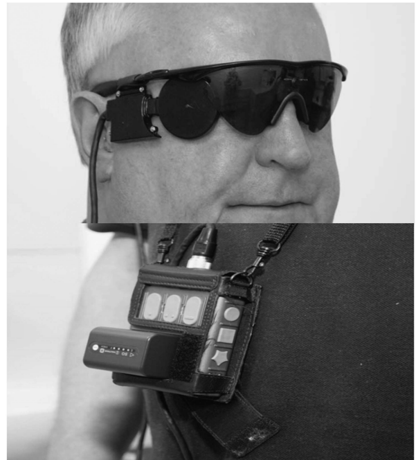
Figure 5 Argus II prosthesis external components. Top image shows the external glasses. The prosthesis consists of an external unit of a pair of glasses mounted with a camera and micro processing unit.
