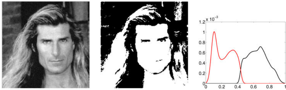
Fig. 12. Left: Fabio image. Middle: Otsu-thresholded Fabio image. Right: intensity distributions for the intensity-normalized image ( I \in [0, 1] ) based on the classes determined by Otsu thresholding.
