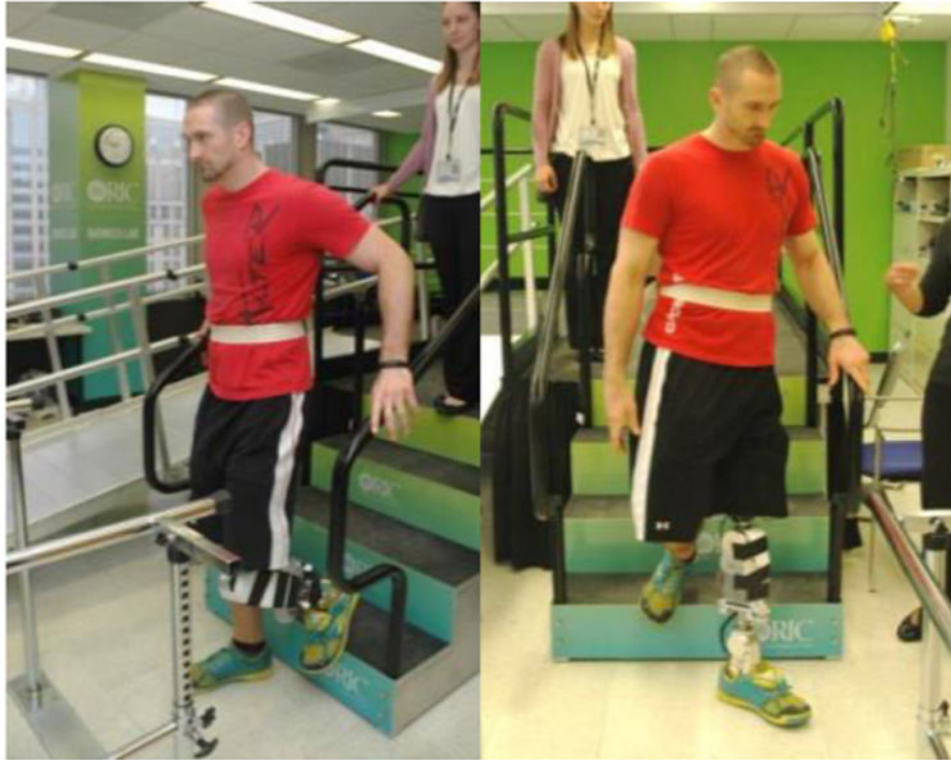
Fig. 2. A transfemoral amputee wearing the powered knee-ankle prosthesis demonstrating various transitions from stair descent to level-ground walking.
