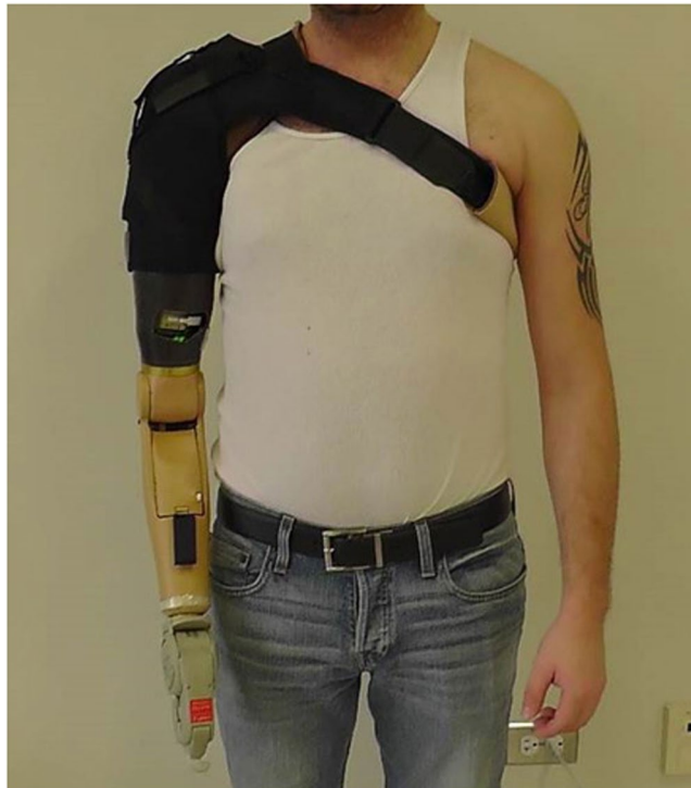
Figure 2. Representative subject wearing the physical prosthesis with a Greifer terminal device (Ottobock, Inc.).
