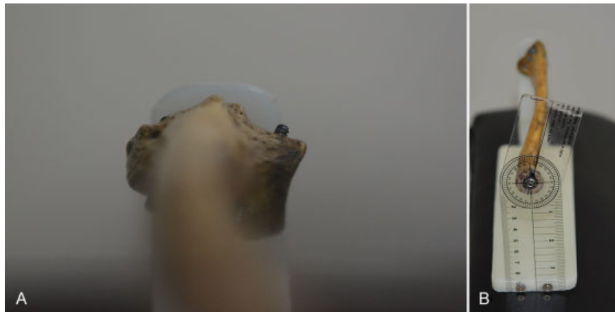
Fig. 2 Figure of jig made for serial oblique views. (A) We set the 90-degree rotation when the Lister's tubercle was in the uppermost position during rotation. (B) The center of the rotatory axis was made at the center of the radial head cartilage. A goniometer was used for valid serial rotation. The supination angle was considered positive.
