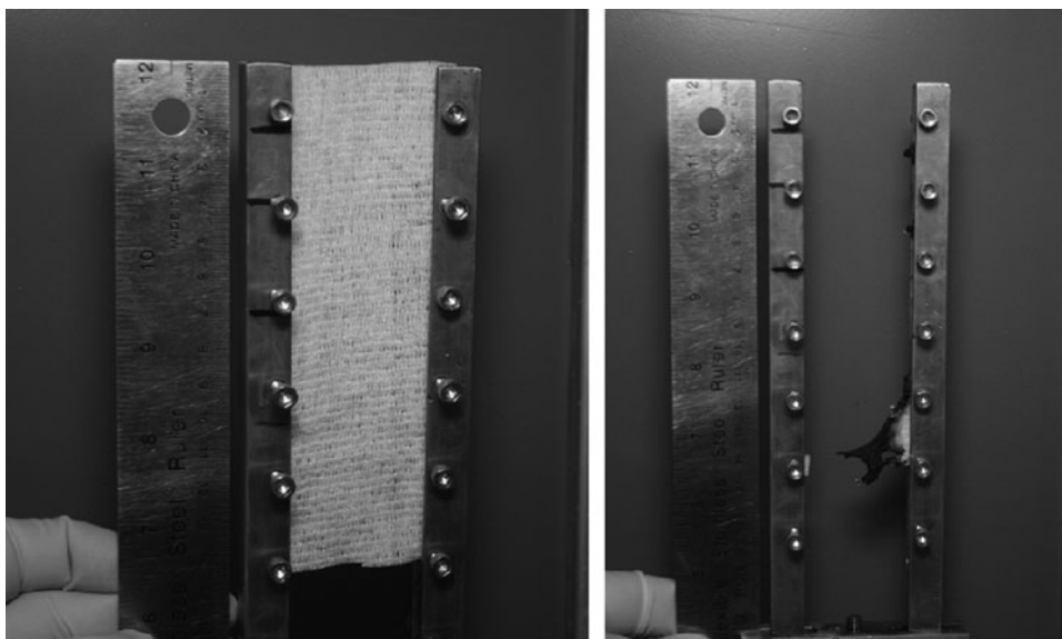
Figure 4. Pre- (left) and post- (right) test photos of gauze, 18% oxygen.
