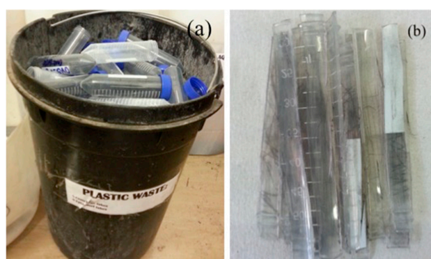
Figure 11. Optical images of (a) the laboratory-based used plastic centrifuge tubes and (b) the washed, dried and chopped used plastic centrifuge tubes.
