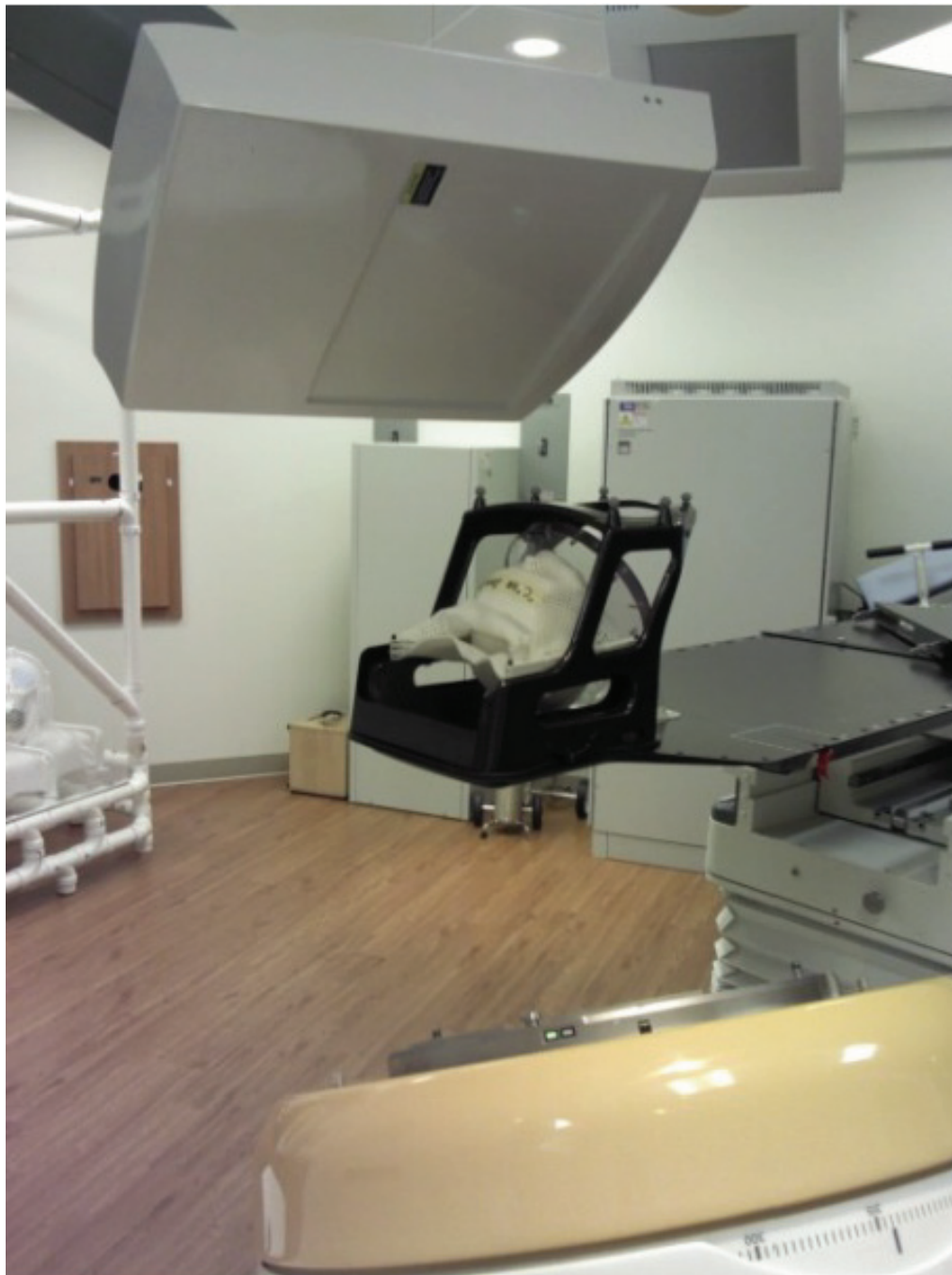
Figure 4. SRS treatment plan delivery with real-time portal imaging acquisition mode with EPID in Novalis Tx linac system. Note that BrainLab Frameless Radiosurgery Positioning Array was used for the initial phantom setup.
