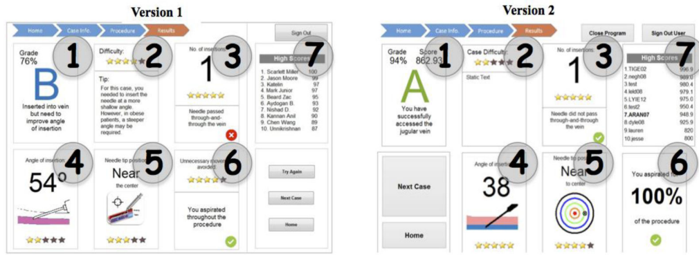
Figure 3. Learning Interface for the Dynamic Haptic Robotic Trainer. Version 1, developed prior to user testing, is shown left. Version 2, with modifications based on user testing, is shown right.
