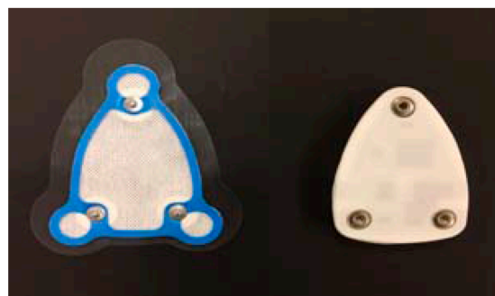
Figure 15. The adhesive coating between sensor and chest.
