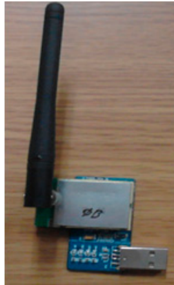
Figure 8. Receiver for the ZigBee communication protocol with a USB interface.
