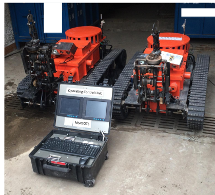
Figure 1. The search-and-rescue robot system used for remote sensing of the underground coal mine environment.
