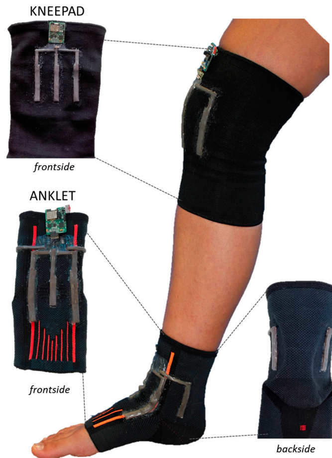
Figure 4. Prototypes of knee and ankle modules each integrating several sensors connected to one read out electronic system that communicates with an external board by a RF module.
