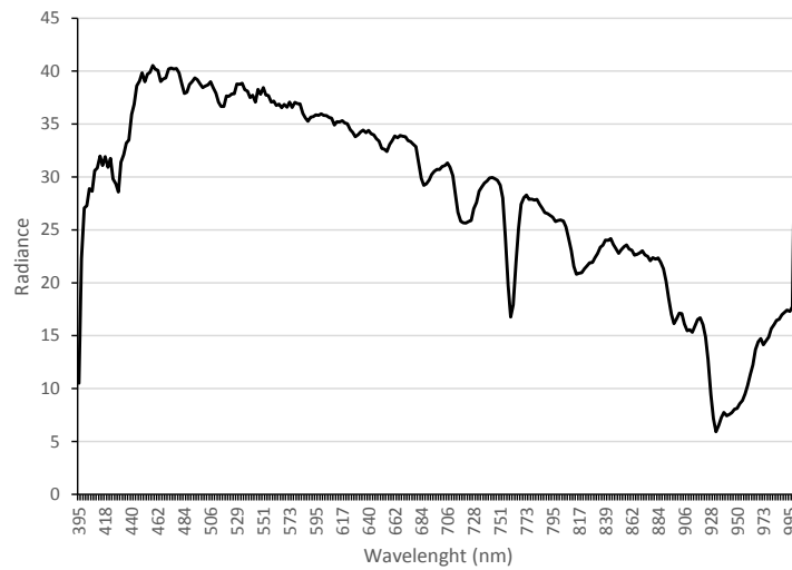
Figure 6. White reference spectrum acquired by the Headwall Nano Hyperspec camera.
