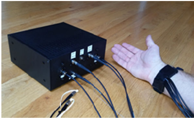
Figure 3. Compact two-channel blood perfusion monitoring system. A fiber optic probe is shown attached to the wrist of a volunteer for scale.
