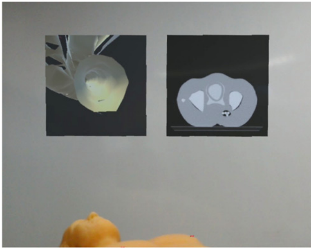
Fig. 3 Two virtual canvasses are hovering above the patient. The left canvas shows the PoV of the catheter inside the vessel and the right canvas renders the representative CT slice in respect to the tracked catheter position
