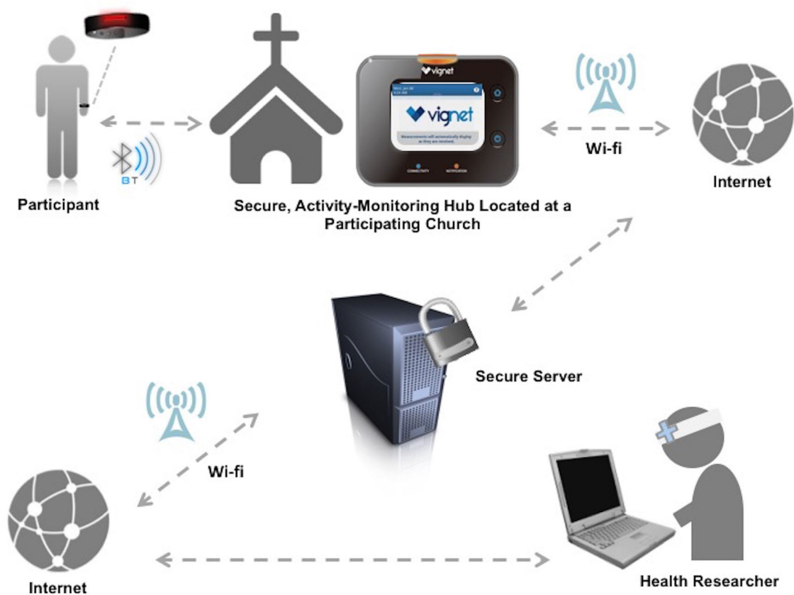
Fig 1 | Secure data collection system for electronic activity monitor data in the Washington, D.C. CV Health and Needs Assessment, (2014–2015)
