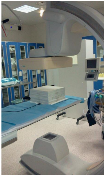
FIG. 1. X-ray equipment in the angiographic room for the in phantom calibration in the reference setting: tube rotation angle at 180^\circ , SSD on the couch of 50 cm (couch thickness 9 cm), and SID 120 cm.
