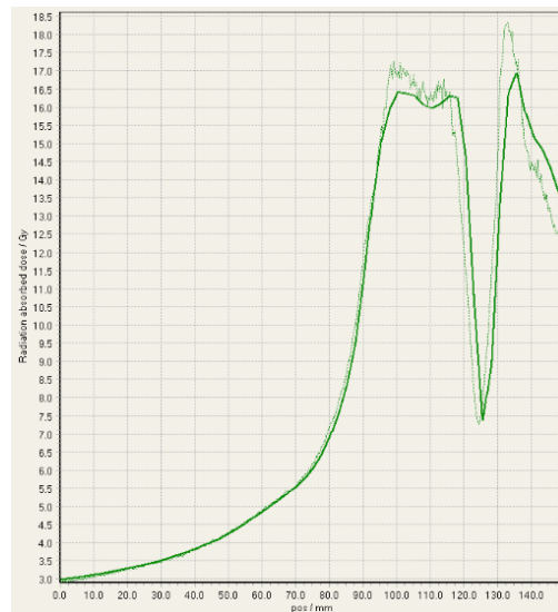
FIG. 6. EBT3 film cross profiles vs. TPS dose maps analyzed in FilmQPro2013 of target volume B delivered on TrueBeam (FFF beam).
