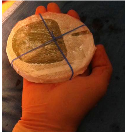
FIG. 7. New shielding setup with the surgical elastic band.
