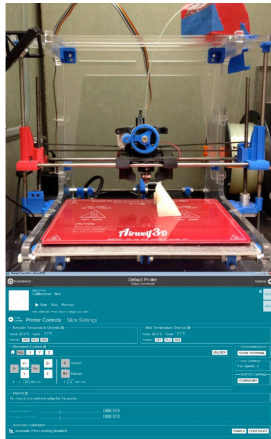
FIG. 2. The Airwolf printer model, XL 3D, is seen above, and the MatterControl Pro software interface can be seen below that. A spool of PLA material is connected to the printer extruder head. An already printed object is shown sitting on the printing bed. During a print, the extruder head would be heating up the PLA filament and depositing, layer by layer, the design exported by the software. The software also controls desired printer and slice settings seen in the screen shot below.
