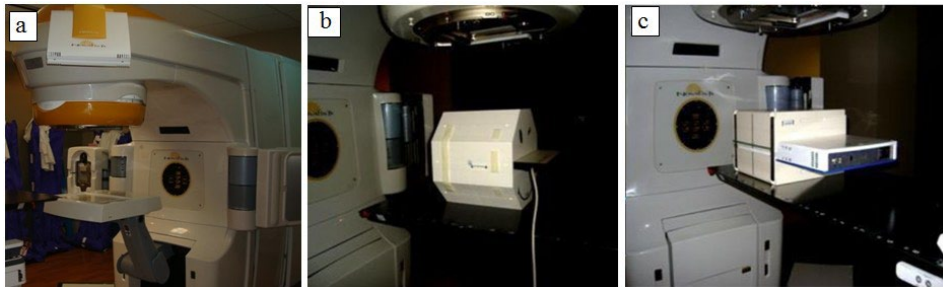
FIG. 3. Picture of the setup: (a) EPID, (b) PTW seven29 array, and (c) IBA I'mRT MatriXX.
