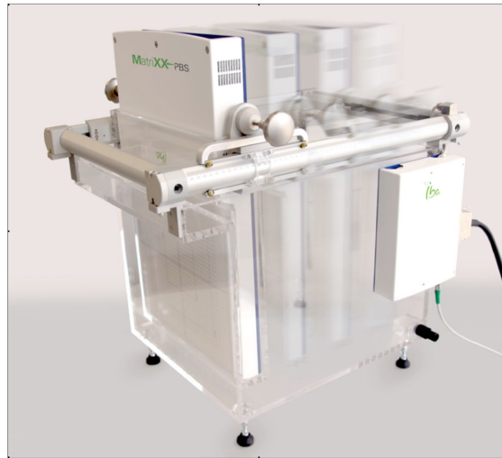
FIG. 1. Setup picture of DigiPhant phantom with beam coming from the left direction and the detector array moving in four locations within the water tank.
