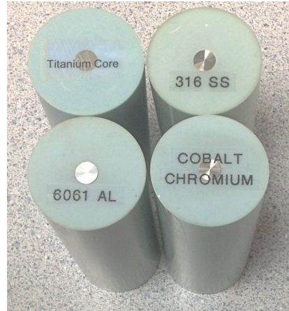
FIG. 2. Custom metal sample plugs designed from plastic-water inserts for the CIRS Model 062 RED phantom. CT number values from these samples were used as data points to characterize the extended CT scale HU to RED conversion curve in the extended range.
