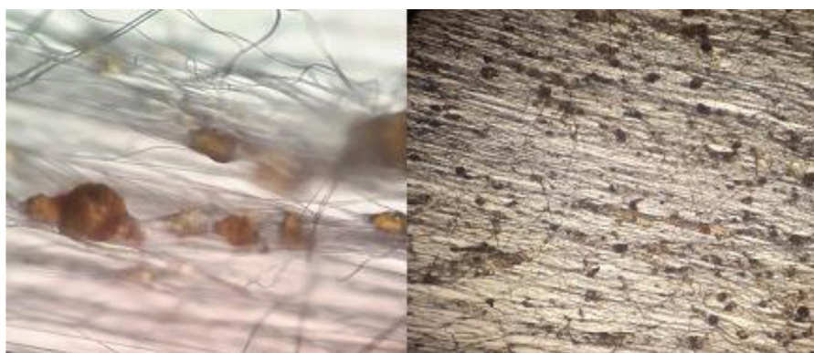
Figure 9: Optical microscope image of sample containing 15% lignin in scaffold
