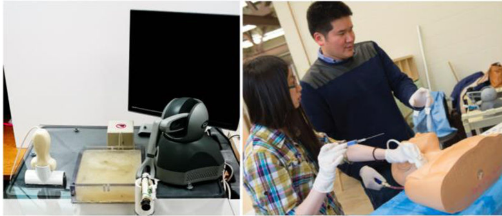
Figure 1. Left - Dynamic Haptic Robotic Trainer. Right – Static Blue-Phantom Gen II Ultrasound Central Line Training Model (Model #BPH660) mannequin
