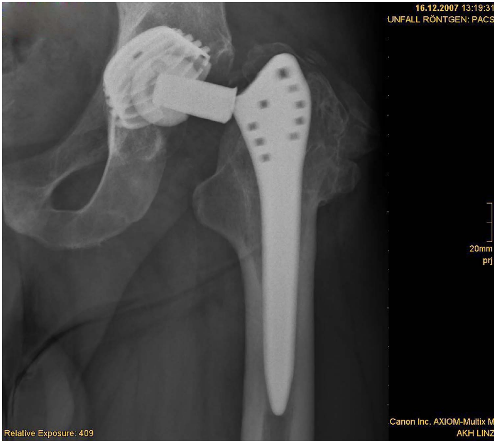
Fig. 6. Radiograph showing implant fracture after 20 years.
