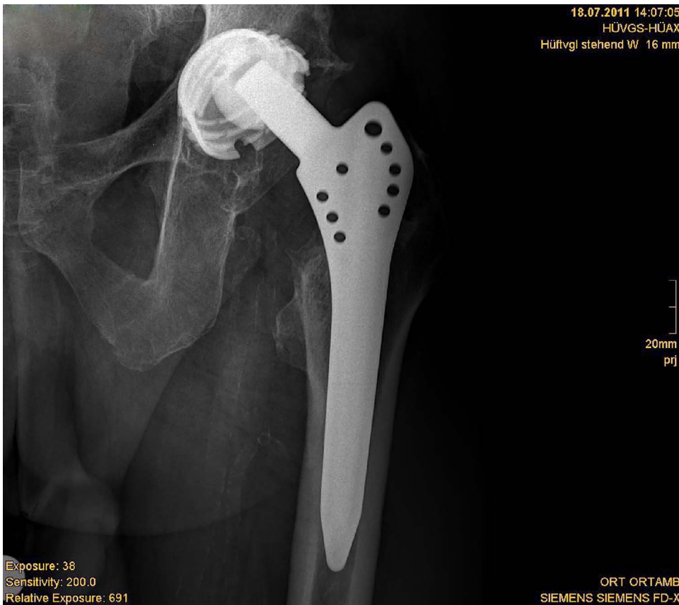
Fig. 7. Radiograph showing totally worn-out liner after 25 years.
