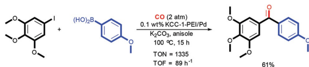
Figure 17. DFNS-PEI/Pd-catalyzed carbonylation Suzuki–Miyaura cross-coupling reaction. Reprinted with permission from Ref. [38]. Copyright 2016 Royal Society of Chemistry.
